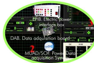
MUAD Power Data Acquisition System
