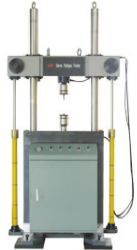
Testing Frame for cap: 50 kN, 100 kN, 250 kN
